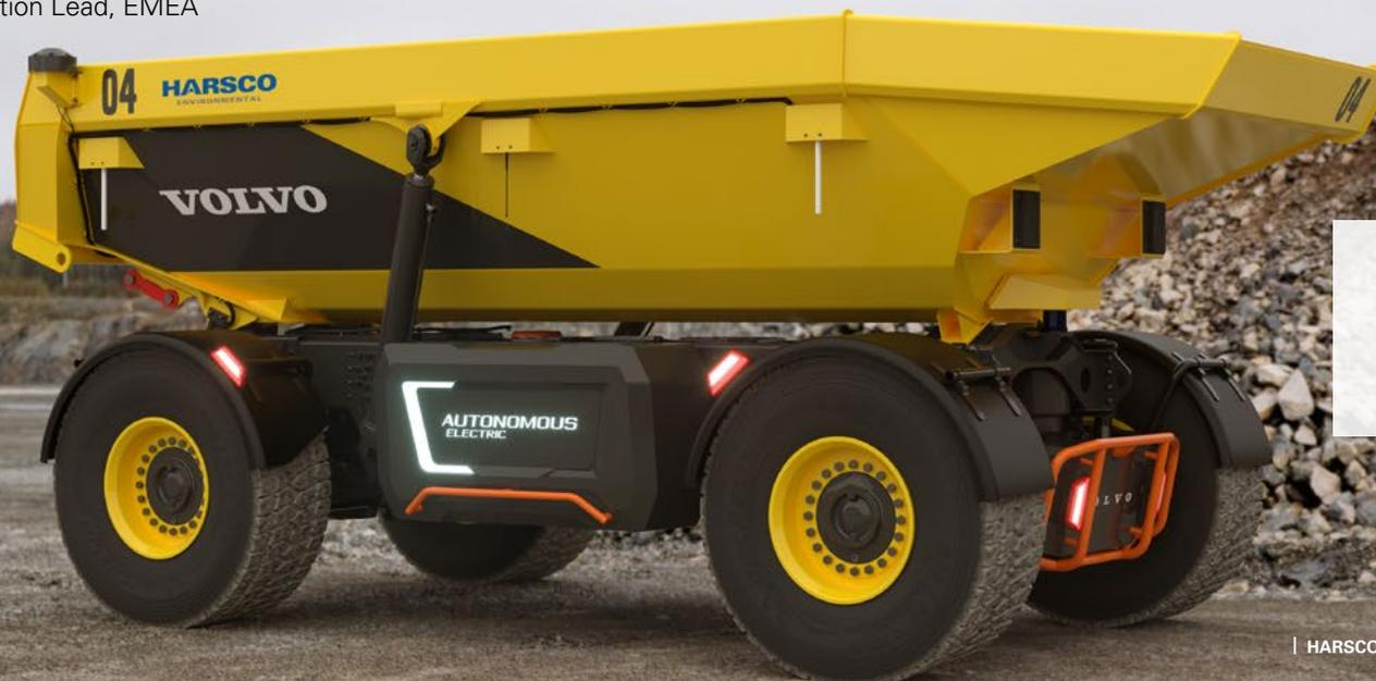
The TA15 uses various sensors, including GPS, light detection and ranging (LiDAR) and radio detection and ranging (RADAR), that allow the hauler to move around the site autonomously.
